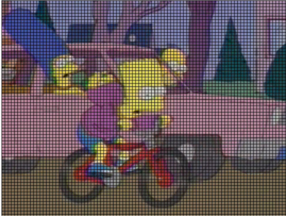
IMAGE 1. VIDEO FRAME DIVIDED INTO GROUPS OF 8X8 PIXELS
